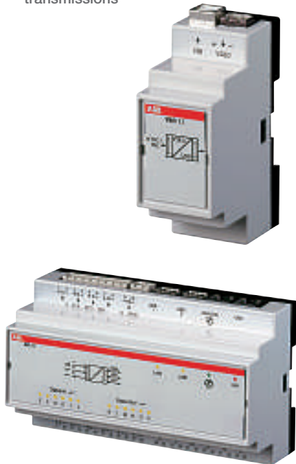
5 First version of the Internet gateway, with four analog and six binary inputs as well as six binary outputs. Target users are owners or occupants of buildings that do not already have a bus system installed.
