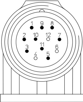
Front view of the signal connector fixed on the terminal box (only for 8C4 and 8C5)
