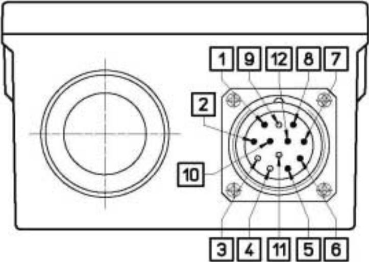
Connection of signal pins on motor side
