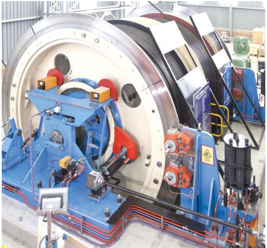
Styldrift: Double Drum Service Winder
