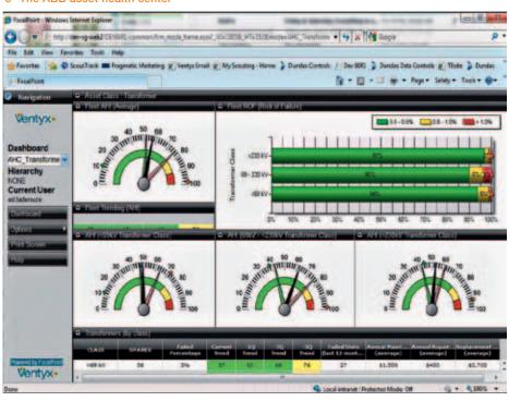
The ABB asset health center combines data from real-time sensor and monitoring devices, as well as from ERP systems and data warehouses.
