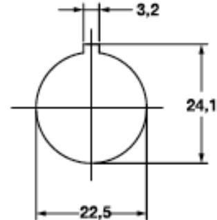
Round front ring OMX\_ for OM - to be specified by Camweb configurator
