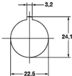
Snap-on key operated handle for OM - to be specified by Camweb configurator
