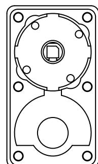
**Key interlocked handle for ON, OL40, OL63 and OL80N, front plate size 64x64, vertical**
