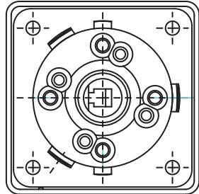
Round padlockable screw mounted handle for OL125 and OL160, type OLZ332R
