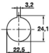
Screw mounted large handle option for ON, OL40, OL63 and OL 80N (type \_ RL \_ )
