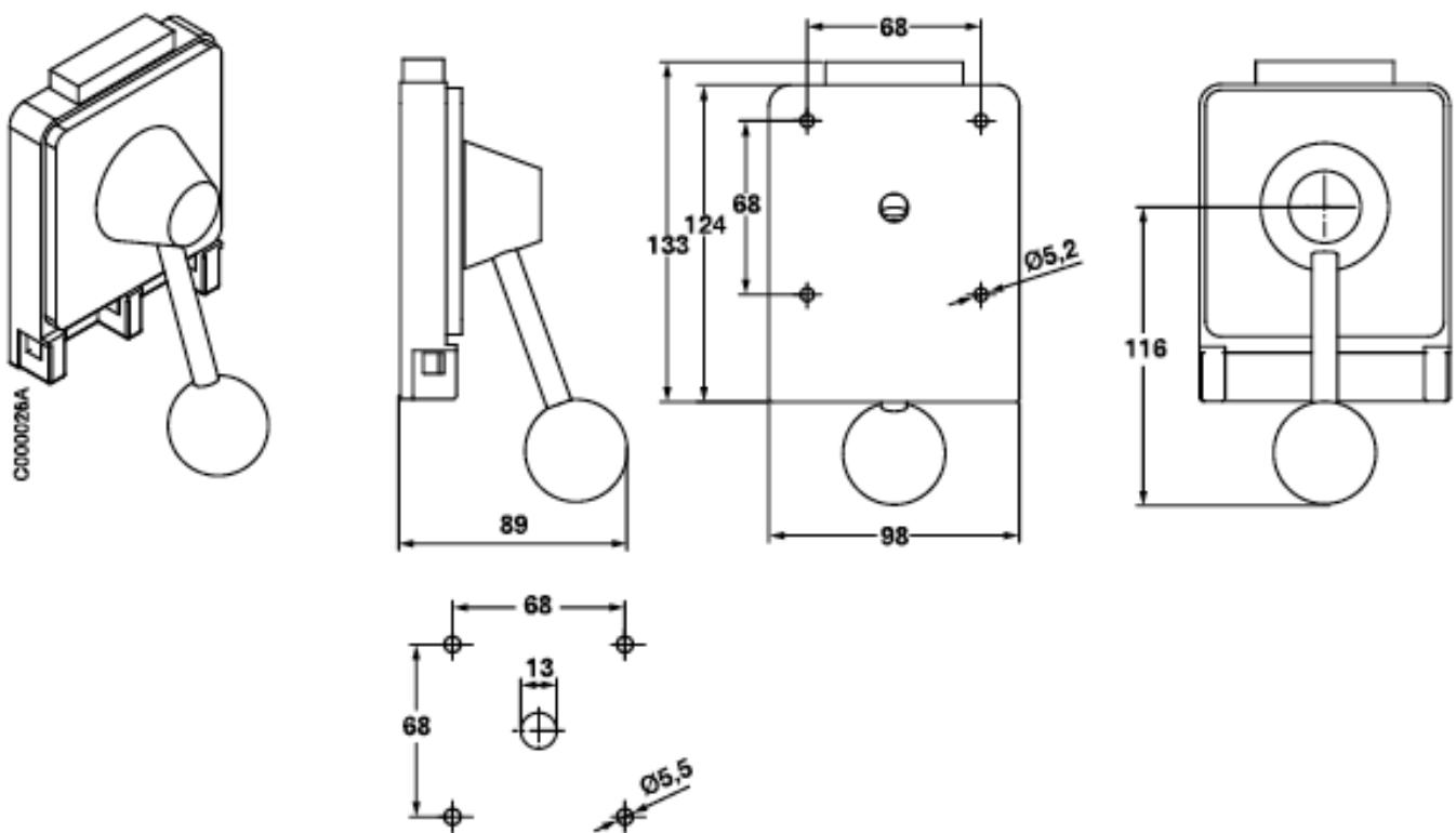
**Key interlocked handle for ON front plate size 48x48, vertical**
