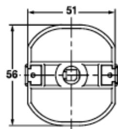
OL40, door mounted with screw mounting handle, type \_RL\_, front plate size 64x64
