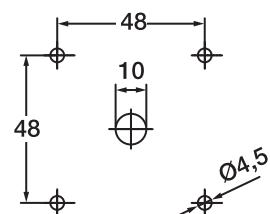
**Double gang (Tandem) drive for OL40, OL63 and OL80 N, standard handle**
