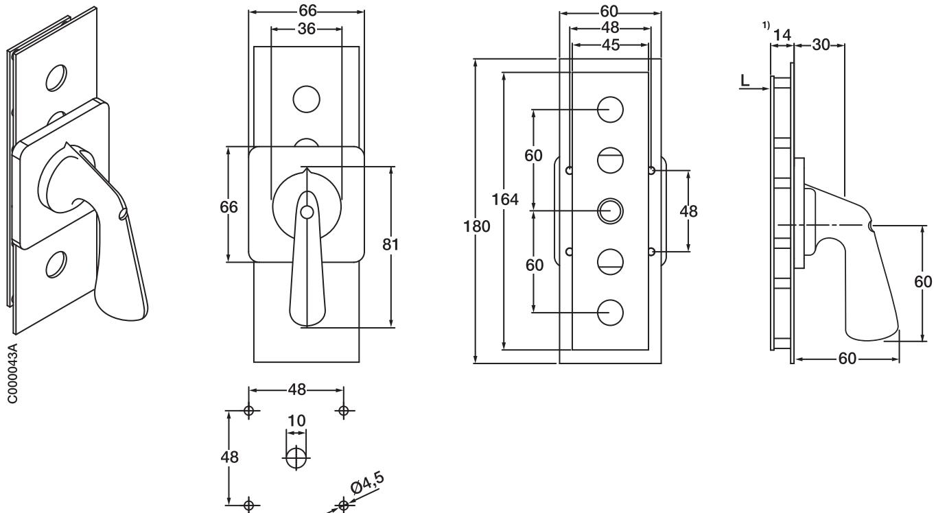
**Triple gang drive for OL40, OL63 and OL80N, standard handle
