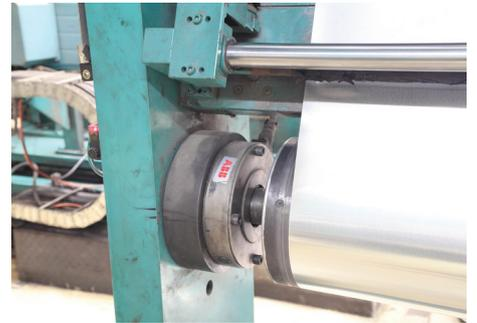
**Pressductor Radial Tensiometers (PRT) in the cold rolling mills and process lines**
