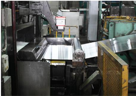
**Millmate Strip Scanner systems in the cold rolling mills**
