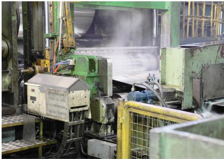
**Stressometer system in the hot rolling mill**
