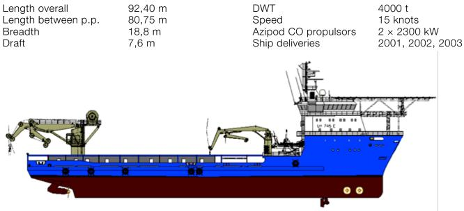
Figure 5-2 Multi functional Platform Supply / ROV Vessel. Normand Rover.
