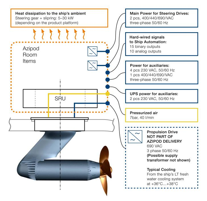
Figure 4-1 Azipod ship interface diagram in a preliminary project format
