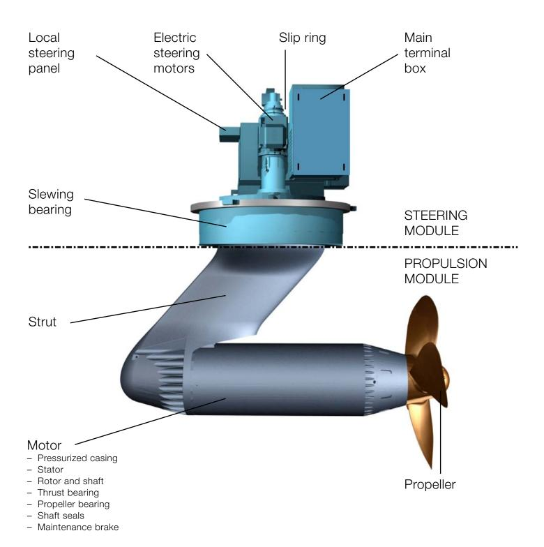
Figure 2-1 Functional elements of the Azipod CO
