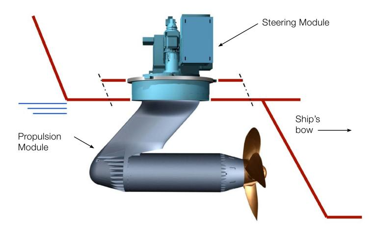
Figure 1-1 Basic arrangement of the Azipod CO
