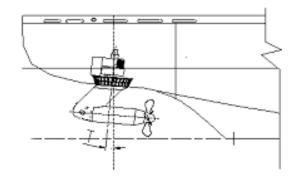
Figure 3-1 Azipod orientation
