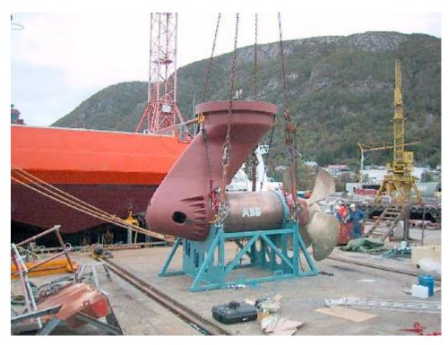
Figure 5-3 Azipod CO1400 propulsor ready for installation at Søviknes Verft.
