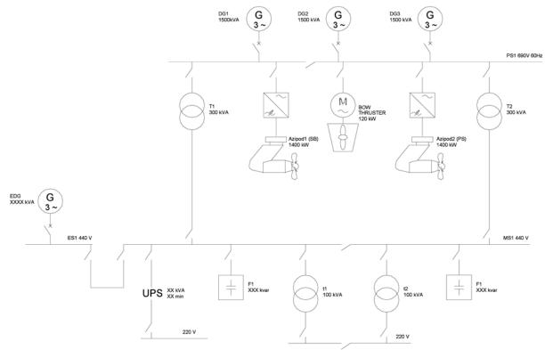
Figure 5-1 Example of a typical electrical power plant
