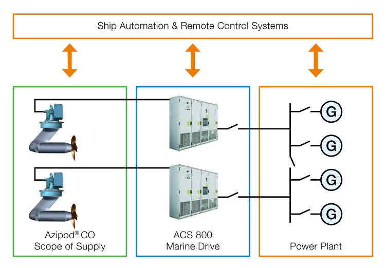
Figure 1-3 Simplified single line diagram of the power plant with a propulsion system.
