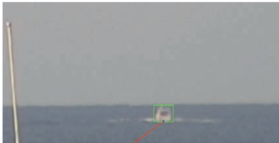
Figure 4: Deep neural network based detection of the 'Medium pleasure craft' at around 9,6 km
