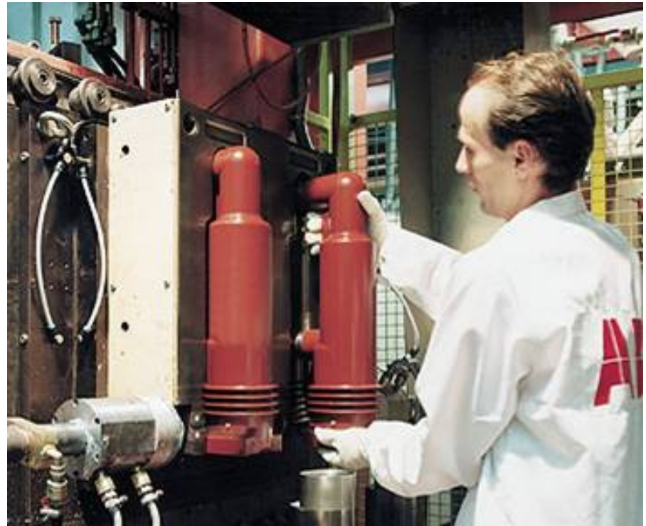
Removal of finished embedded poles from the mould
