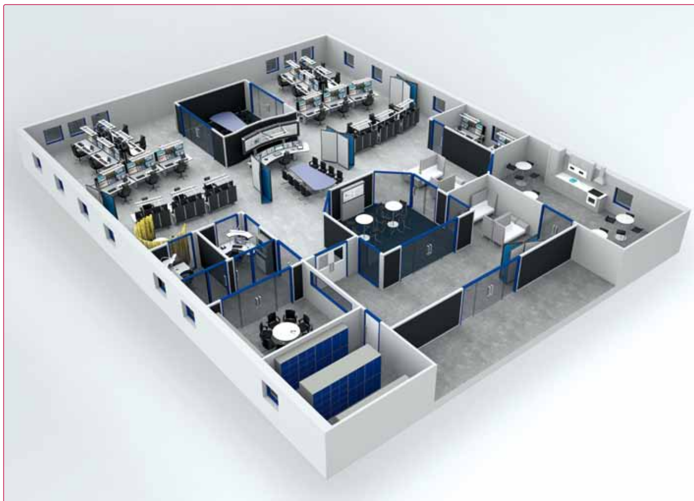
An example of a crane operations control room layout based on experiences from process industries. In addition to the operator workstations the layout takes into consideration the positioning of adjacent areas such as meeting rooms, locker rooms, and dining areas.
