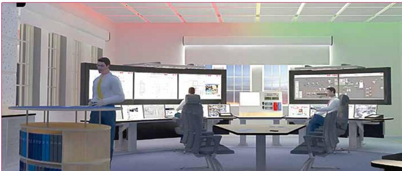
Lighting can be used to support operator in critical operational situations. In this example from process industries, the surrounding lighting is tuned down to increase operator's concentration on the screens. Lights in different colours are used to communicate to others in the room that the operator is handling a critical situation (red light), so is reminded not to disturb the operator.
