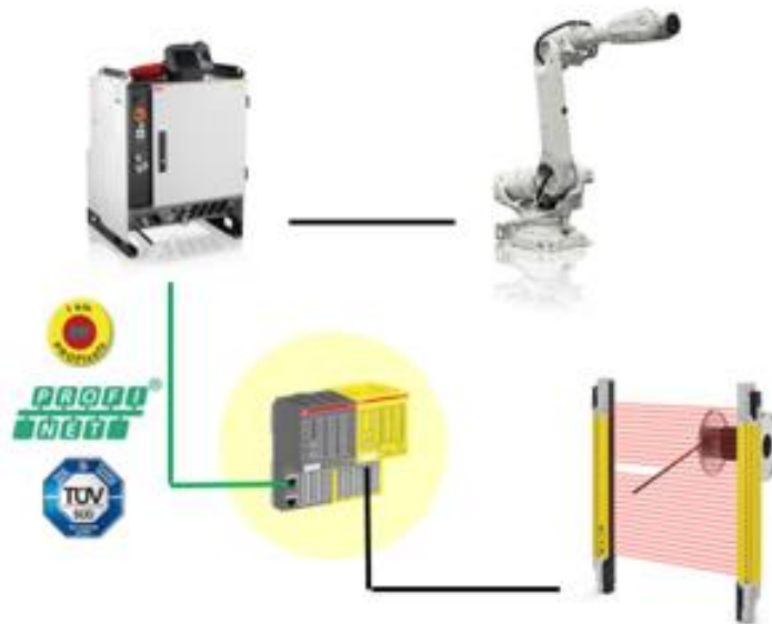
Fig. 1: IRC5 controller with SafeMove2 and ABB safety I/Os configured using the “Prepared for ABB CI502” option
