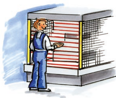
Light curtain for short safe/minimum distances
