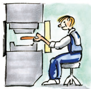
Light curtain to protect during cycle initiation
