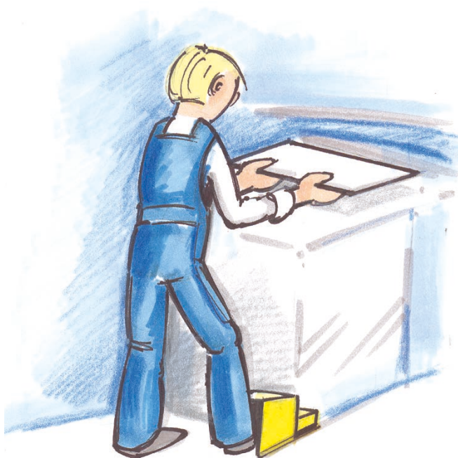
Safety foot operated switch with three-position function.
