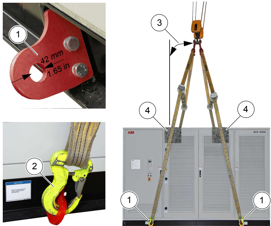
Fig. 4-1 Transporting the cabinet by crane
