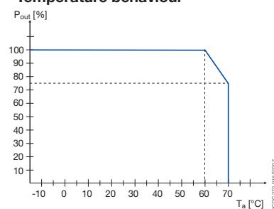
Characteristic curve of temperature at  $U_{\text{OUT}}$
