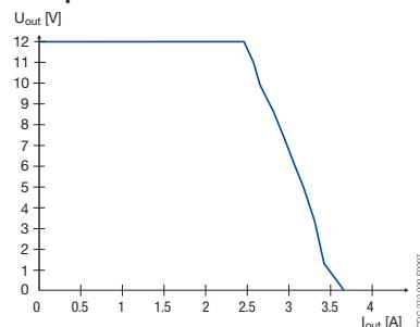
Characteristic curve of output at  $T_a = 25 \text{ } ^\circ\text{C}$
