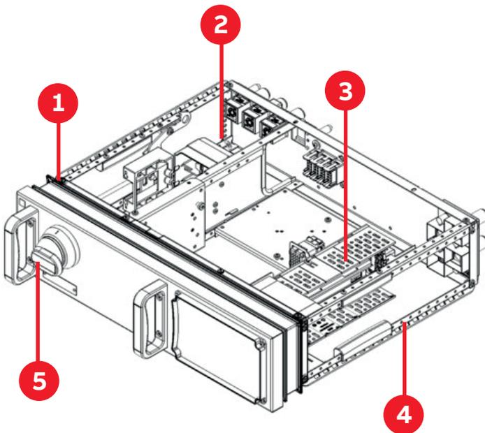
Whether the module is small, medium-size or large they all connect directly to the laminated bus plate. There is no need for special conductors simplifying the conversions of compartments when needed.
