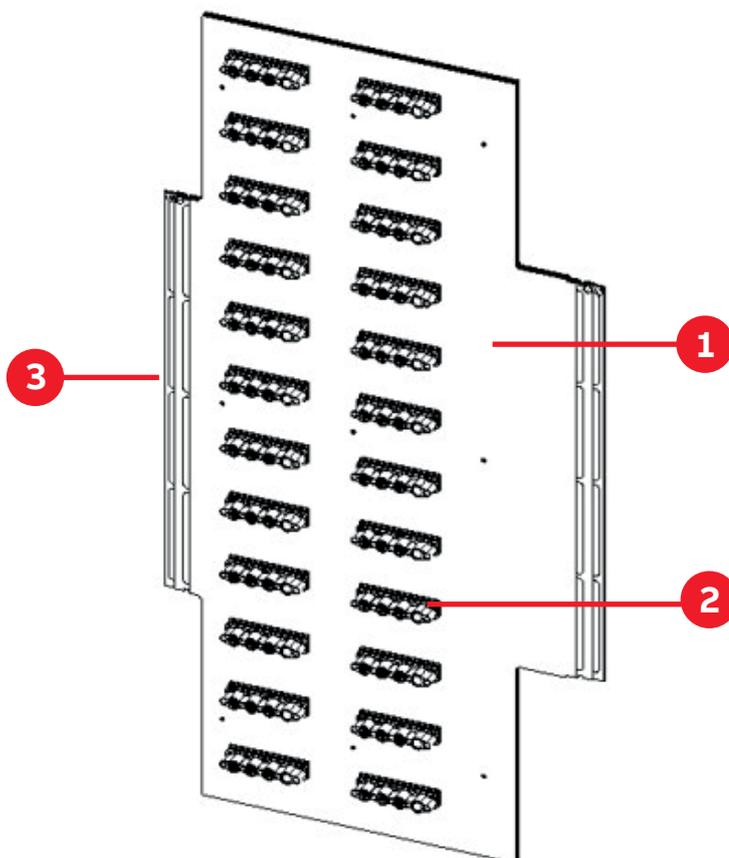
1. The copper phase plates are fully segregated by a solid insulation material. The insulation material is a Sheet Molding Composite (SMC) consisting of glass-fiber reinforced polymer material, halogen-free, flameretardant and self-extinguishing. This design makes it impossible for an arc to pass between phase plates or between equipment compartment and cable compartment.
