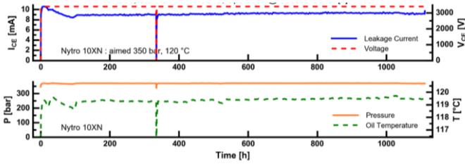
Figure 5: The HTRB measurement shows in the first graph the applied voltage and the measured leakage current vs. time, where in the second plot the oil temperature and the pressure are indicated as well, respectively
