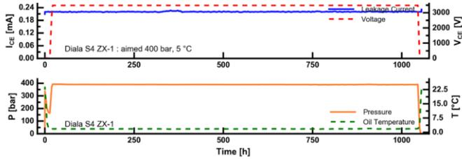
Figure 6: The LTRB measurement shows in the first graph the applied voltage and the measured leakage current (offset on Ice values) vs. time, where in the second plot the oil temperature and the pressure are indicated as well, respectively
