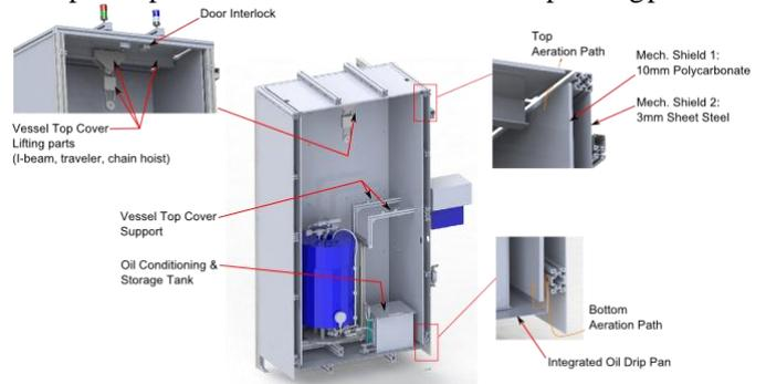
Figure 1: Drawings of the cabinet with the pressure vessel in blue showing the safety features, electrical safety circuit allow for voltage application only in case of closed cabinets.
