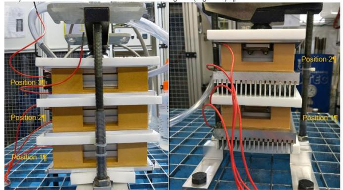
Figure 4: StakPak submodules assembly for 3 submodules for LTRB (left side) and for two submodules HTRB (right side)
