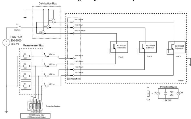
Figure 3: Electrical diagram for testing of IGBT chips (here for three StakPak submodules)
