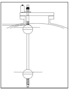
(if the float is clear to enter the man-way nozzle). Adjustment of the upper spring location by the customer will alter the gauging span and may expose the float to damaging contact with the tank sides.
