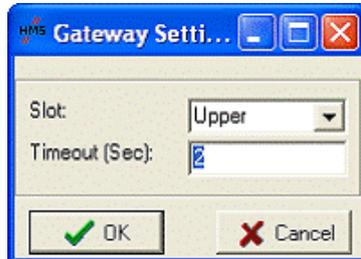
Now with the network online, all devices may be configured. To configure the Anybus-M DEV, double click on the device and click yes to synchronize the parameters. The gateway must be in Idle mode in order to make any changes, select Idle and click download.
