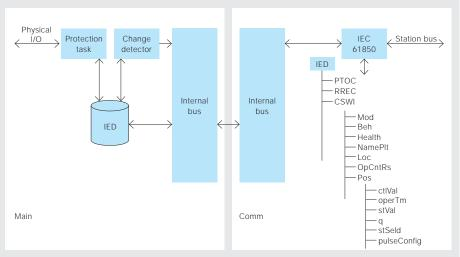
5 IEC 61850 handling in case of a separate communications module
