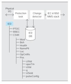
In IEC 61850-based architectures, conventional wiring has been eliminated and binary and analog signals are transmitted and received via the communications interface.
