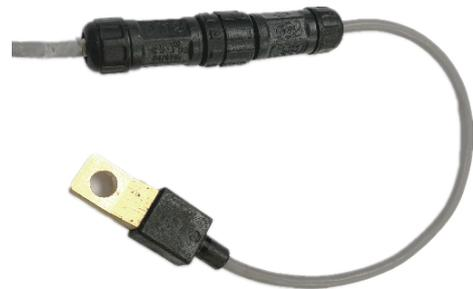
(b) Connection between sensor probe and gray box
