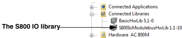
Figure 49. The new S800IO library has been connected to the controller
