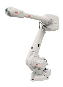
IRB 4600 is a highly productive general purpose robot optimized for short cycle times where compact robots can help create high density cells. The IRB 4600 enables more compact manufacturing cells with increased production output and higher quality - and that means improved productivity.
