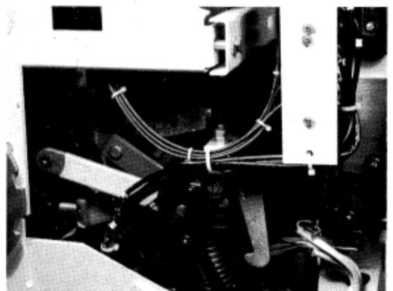
Figure 3-11. Relocated Terminal Block and Wire Harness
