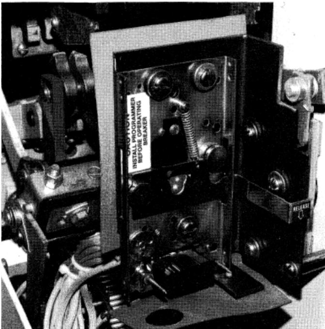
Fig. 3-17. Programmer Plate Installation
