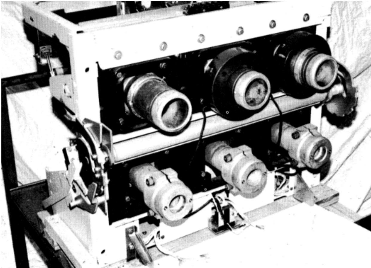
Fig. 4-5. Phase Sensor Installation for AK-75, AK-100 Breakers
