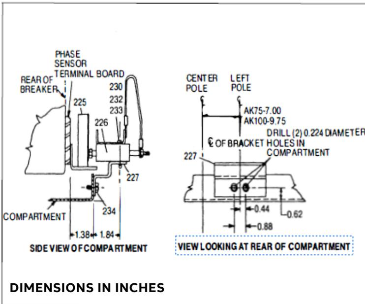
Fig. 6-1. AK-50, AKS-50 4th Wire Disconnect Type AKO
