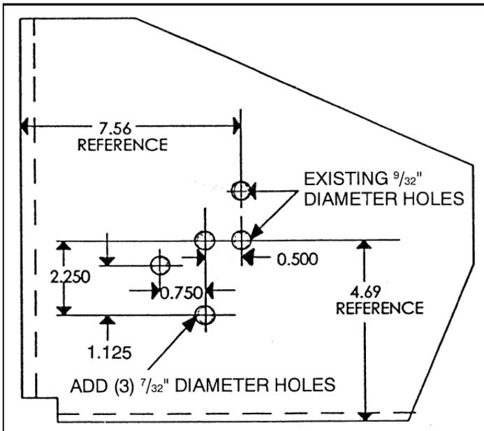
Fig. 3-4. Mounting Hole Pattern
