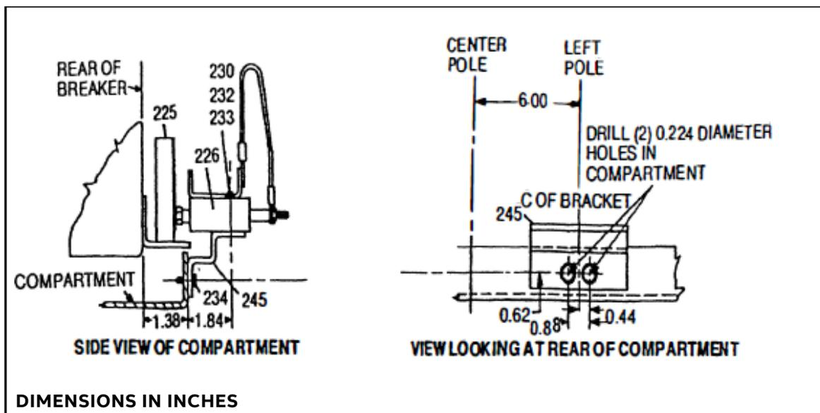
**Fig. 6-5. 4th Wire Disconnect Installation Types AKD-5, AKD-6**
