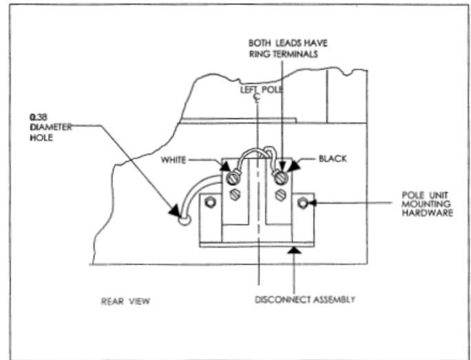
Fig. 5-2. 4th Wire Disconnect Installed Types
