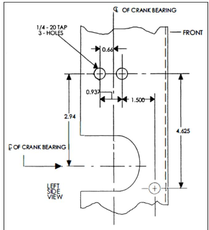
Fig. 3-16. Mounting Plate Hole Pattern
