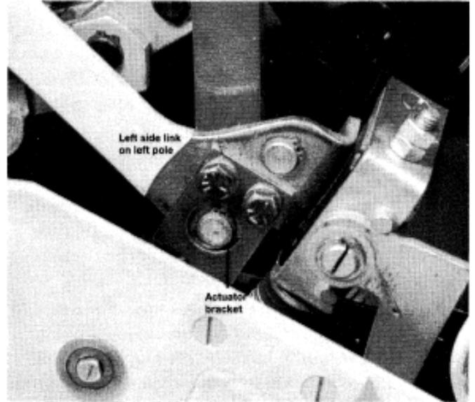
Fig. 4-1. Flux Shifter Actuator Bracket Installation
