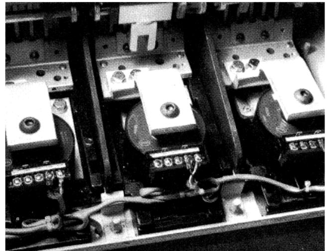
Fig. 4-4. Phase Sensors and Harness Installed
