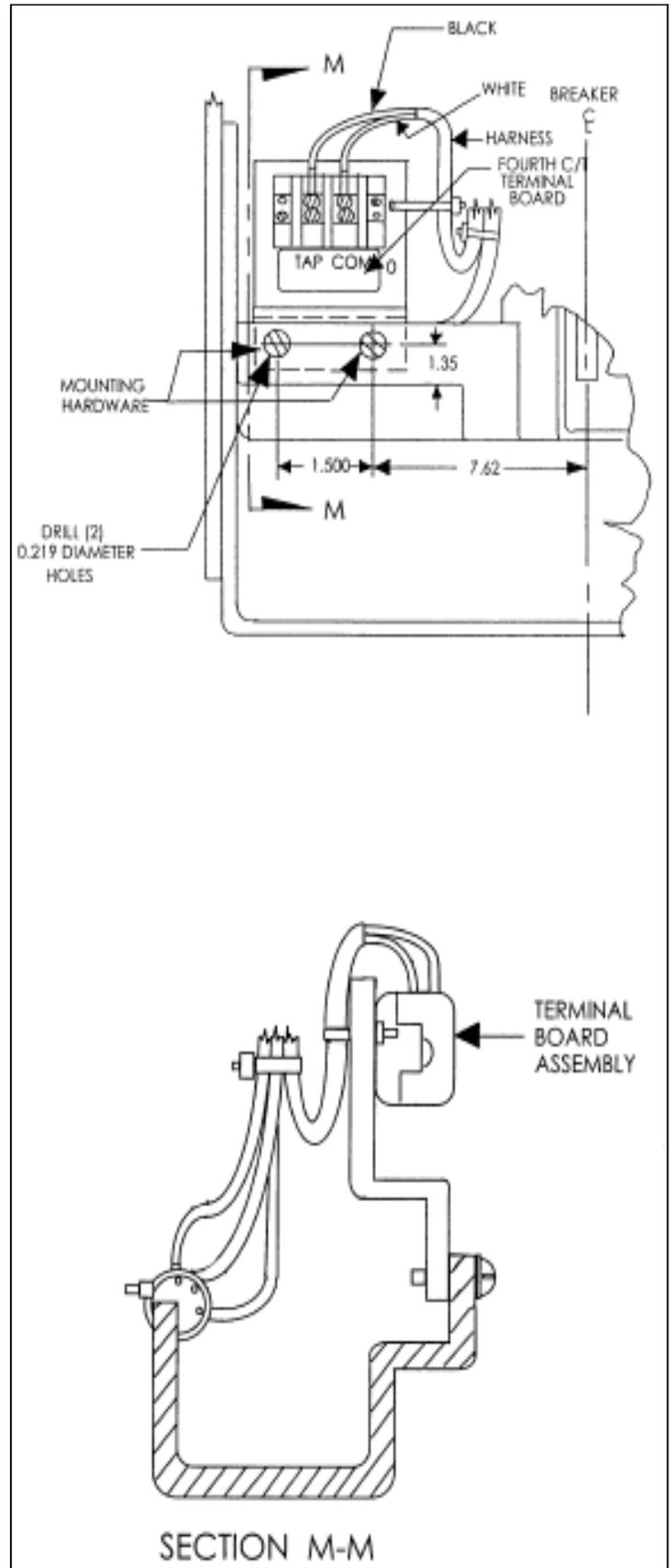
Fig. 5-1. 4th Wire Terminal Board Installed Types AK-50, AKS-50 Stationary
