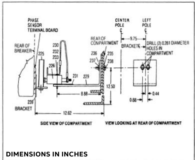
**Fig. 6-3. AK-100 4th Wire Disconnect Type AKO**
