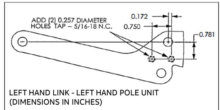
Fig. 4-2. Actuator Bracket Mounting Holes
