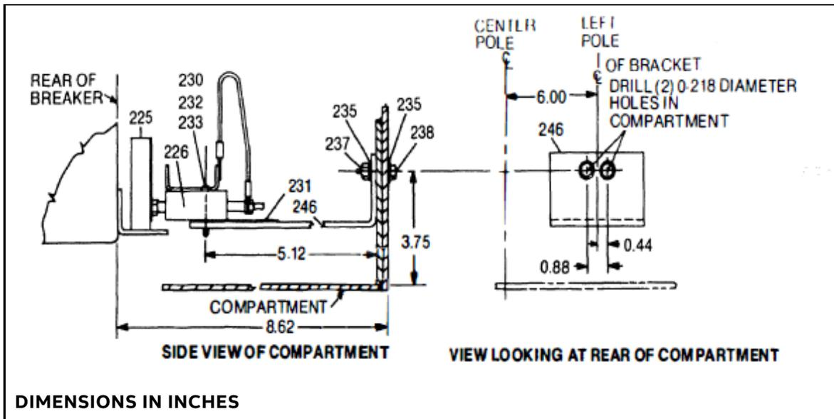
**Fig. 6-4. AK-50, AKS-50 4th Wire Disconnect Type AKO**
