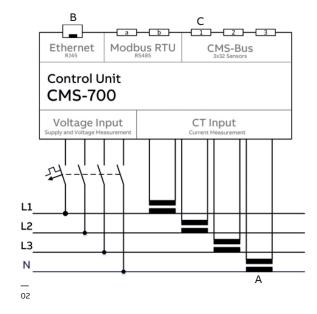
Mains current transformers (CTs) [A] measure the phases L1, L2, L3 with optional N and are connected to the CMS-700 Control Unit inside the master tapoff unit. An RJ45 or RS485 interface [B] is available to read out the measured values. The three CMS buses [C] on top of the Control Unit are wired out of the master box to RJ45 sockets. From there each of the three buses is daisy-chained to the subsequent slave tap-off units with open-core sensors.
