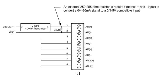
The input range is 0-10.34 volts for the three 0-5V analog inputs (Al1, Al2 & Al3). The inputs have a low-pass filter -3dB point of 100Hz. Sourcing Device must be capable of driving 10K input impedance.
