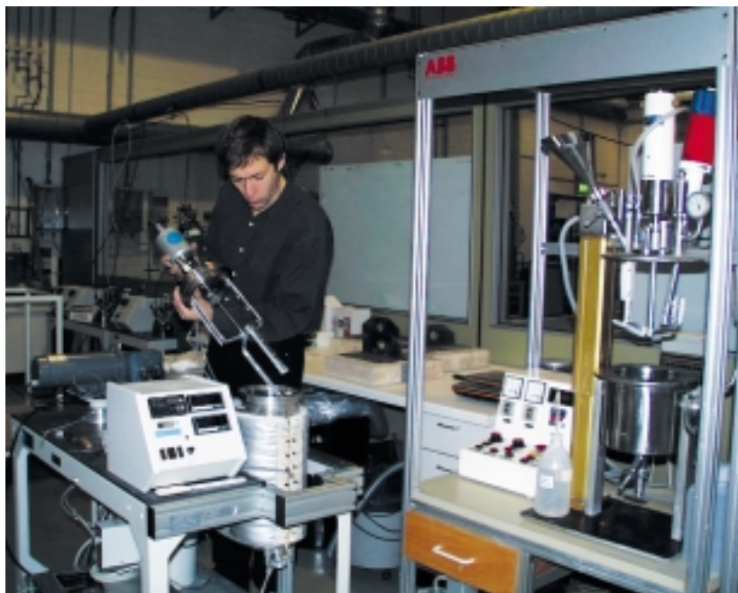
3 Equipment at ABB Corporate Research in Heidelberg for scale-up of the novel zeolite synthesis method at kilogram level
