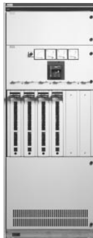
Switch-fuse in the supply cubicle. Due to breaking on both sides fuse replacement always takes place when the unit is dead. The door is interlocked and can only be opened when the switch is in the closed position.
