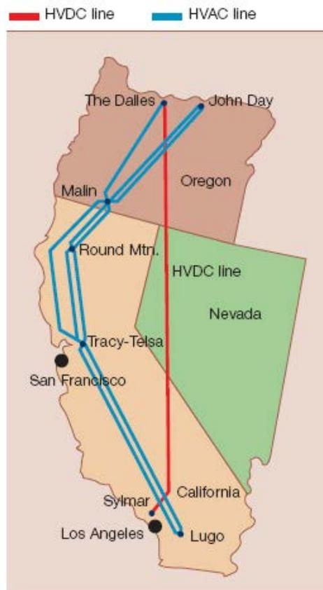
Figure 1 The Pacific HVDC Intertie with parallel ac lines.
