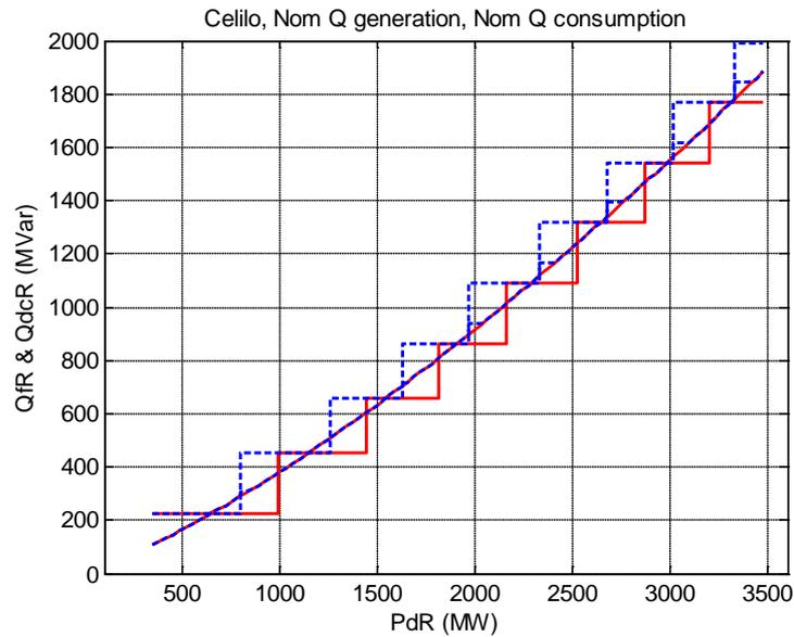
Figure 3 Celilo upgrade Reactive power control
