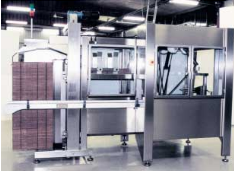
11 Incorporated in a FlexWrapper™ packaging machine, an IRB 340 picks and places finished, customized cartons.
