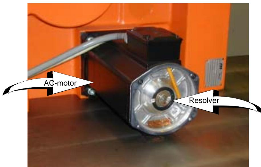
Figure 14 Motor with resolver
