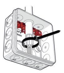
Make sure that the cable tie is secured around the strain-relief before tightening the cable tie. When the cable tie has been tightened and the installation is complete, make sure that the strain-relief is secured by pulling firmly at the cable in an outward direction.
