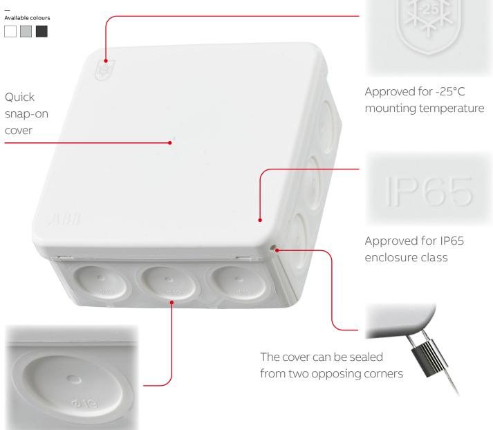
Includes 14 (Ø 19 mm) membrane cable entries. 3 on each sides and 2 at the bottom. The entries include markings for the maximum cable size.
