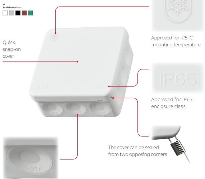
Includes 14 membrane cable entries, 3 on each side (Ø 17 mm) and 2 at the bottom (Ø 19 mm). The entries include markings for the maximum cable size.
