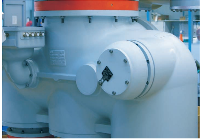
Current transformer in split-up module
