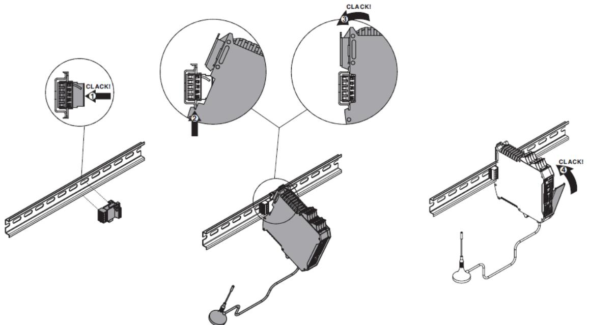
Connect the antenna cable to the SMA antenna connector and make sure that the place where the Ekip GPRS-M is installed is covered by GSM signal. Insert the SIM card in the corresponding slot.
