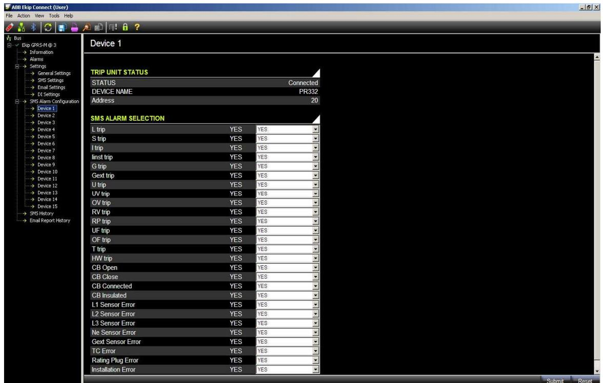
In this page user can enable/disable the event that triggers the alarm SMS for the selected TU (one page for every trip unit is provided). The page contains all the available events that can be generated by the trip unit and that can be managed by Ekip GPRS-M.
