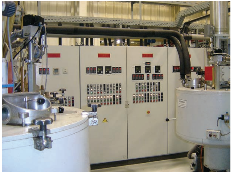
Computer controlled epoxy mixing for exacting consistency.
