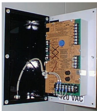
Winding Temperature Indicator provided with isolation barrier.
