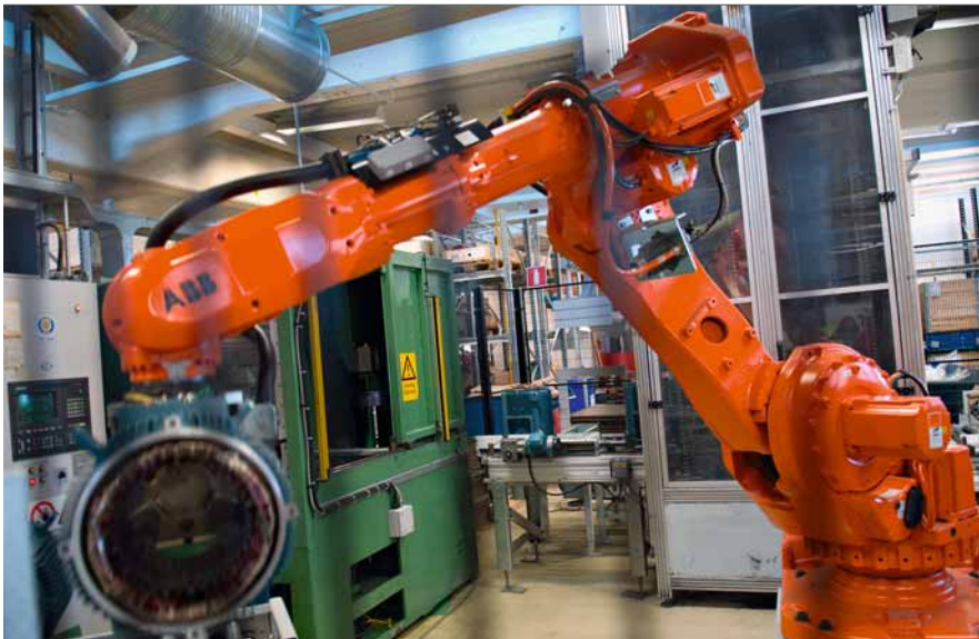
3 Heavy lifting by an IRB 6600
