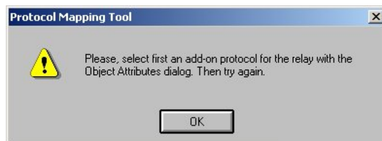
Fig. 3.4.1.-1 Message shown during startup of the Protocol Mapping Tool, when no add-on protocol has been selected.
