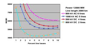
Fig 4. Cost comparison: 800 kV AC, 1,000 kV AC, 500 kV DC and 800 kV DC. [Ref 3].
