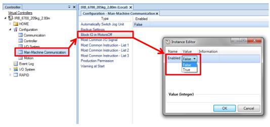
The setting disables the FlexPendant and RobotStudio buttons for changing I/O signals on a real controller. For a virtual controller, the setting is ignored by RobotStudio.
