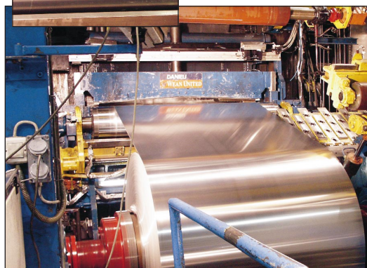
MTG in action at the uncoiler side in the Sapa mill. Note the layer of coolant in the measuring gap.
