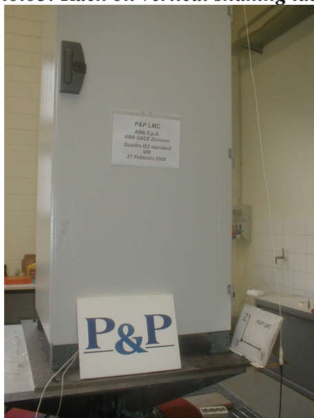
Photo5: Rack on vertical shaking table
