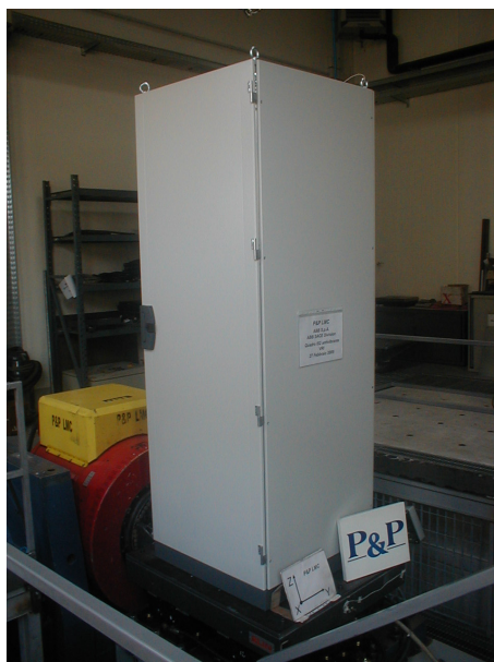
Photo6: Rack on horizontal shaking table
