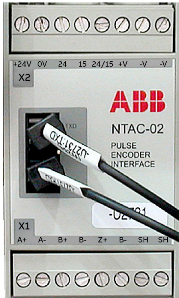
Figure 35 – NTAC-02 pulse encoder interface
