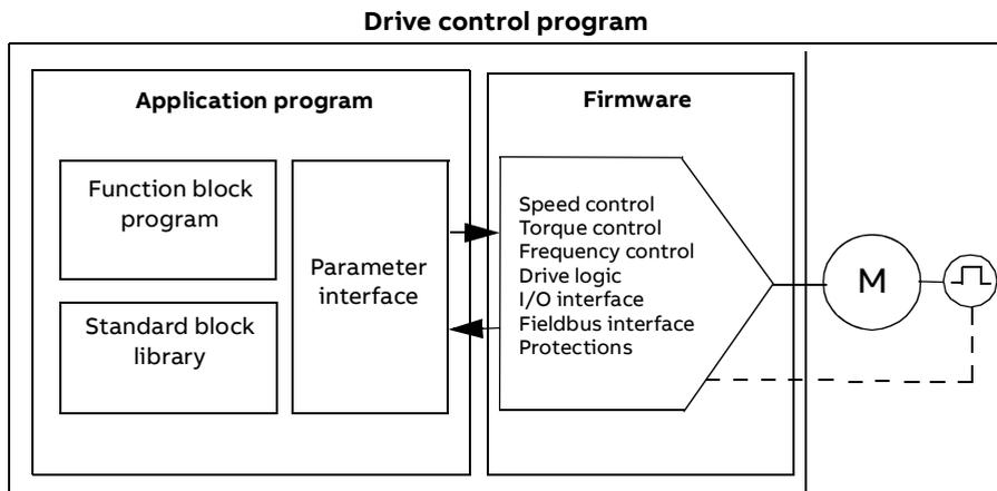
The firmware program performs the main control functions, including speed, torque and frequency control, drive logic (start/stop), I/O, feedback, communication and protection functions. Firmware functions are configured and programmed with parameters.
