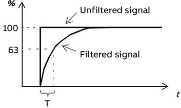
$O = I \times (1 - e^{-t/T})$ <p>I = filter input (step)<br/> O = filter output<br/> t = time<br/> T = filter time constant</p> <p><b>Note:</b> The signal is also filtered due to the signal interface hardware (approximately 0.25 ms time constant). This cannot be changed by any parameter.</p> | 0.100 s              |
