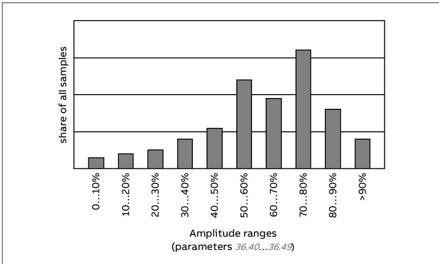
Amplitude logger 1 is fixed to monitor motor current, and cannot be reset. With amplitude logger 1, 100% corresponds to the maximum output current of the drive ( $I_{\max}$ ). The maximum output current values are listed in the section
