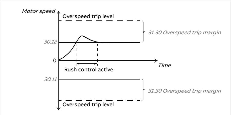
The function is based on a PI controller. The program sets the proportional gain to 5.0 and integration time to 2.5 s.
