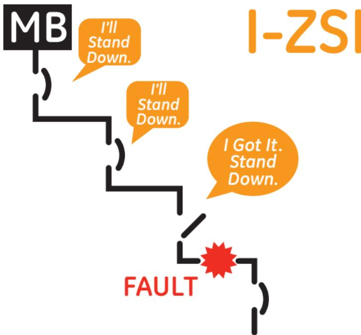
These simple diagrams represent how the breakers communicate using I-ZSI or WFR to simultaneously provide selective coordination and arc flash mitigation.
