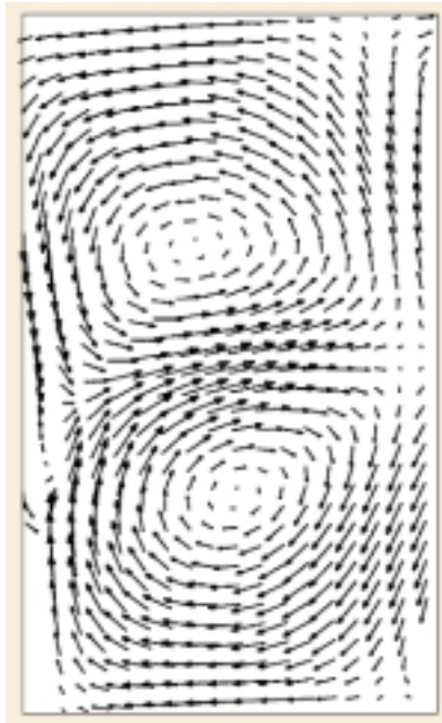
Computed secondary flow patterns at the fuel injection plane (half channel width) 12
