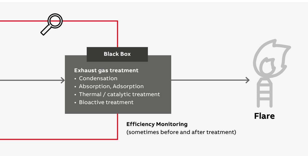
The method chosen depends on the VOC load in the off gas. If VOC concentration reaches vol% levels condensation is the method of choice. Highest efficiency is achieved with thermal or catalytic combustion. But all pollution control systems might require a TOC measurement from lower ranges to higher levels but must not exceed the lower explosive limits.
