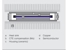
10 Cross-section of a HiPak IGBT module
