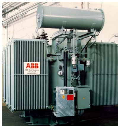
Figure 3.16: A mineral oil-insulated 16 MVA 66/11 kV distribution power transformer ready for despatch at factory
