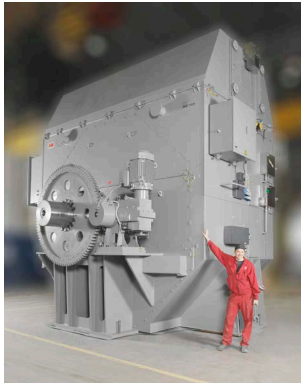
Figure 3.71: Reciprocating compressor motor 24 MW
