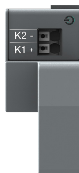
Fig. 5.8 Signals of auxiliary power supply module OXE1
