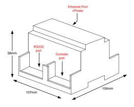
Free space recommended to install the device into a cabinet (wall or DIN rail mounting), with space enough for external connections:
