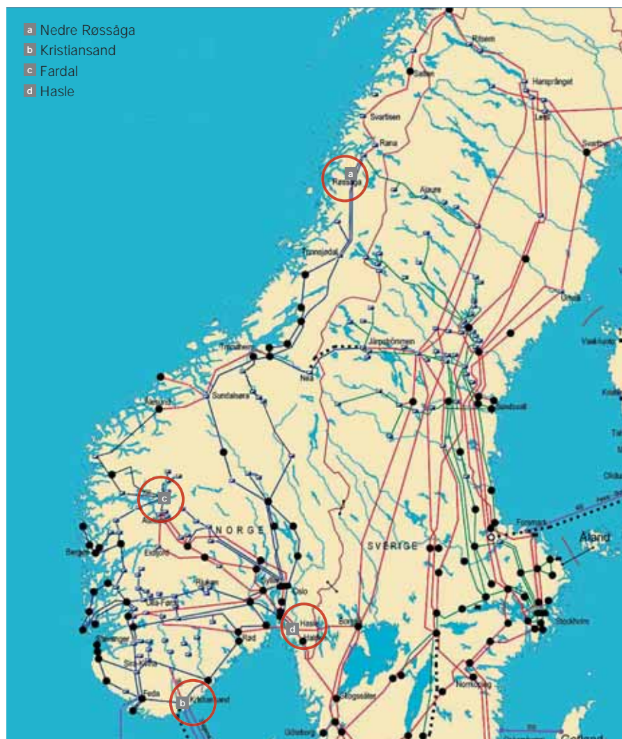
1 The Nordic transmission grid and installed PMUs, indicated with red circles
